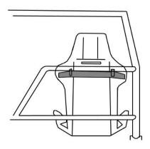
You may fit a Head Restraint Net on the on the safety fence side of the race car only. A quick release window net must be fitted to the driver's door window aperture and must be of quick release/cloth type only. Net spacing must be 76mm x 76mm maximum.
